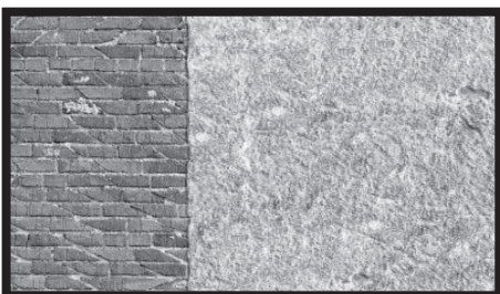
Fig.43 - For wall installation on exterior plaster, KERLITE 3plus and KERLITE 5plus must be adhered onto a high performance substrate, which resists mechanical stress, such as structural movements, the weight of tiles, any thermal expansion and atmospheric agents. In this case, we recommend plaster such as KR100 from Fassa Bortolo or BF02 from Grigolin , or any plaster having the same characteristics with an average adhesion capacity to brick of at least 1 N/mm 2 (approx. 10 kg/cm 2 ). In correspondence with the edges of doors, windows, etc., it is recommended to apply strips of mesh on the plaster, such as Mapegrid G 120 from Mapei , positioned at 45°. During installation, pay attention to stringcourses and structural joints.
